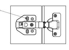
To adjust the height position of the door loosen the screws indicated on the side panel bracket, you will need to do this on all the brackets, adjust the door position and retighten the screws to secure the door.
