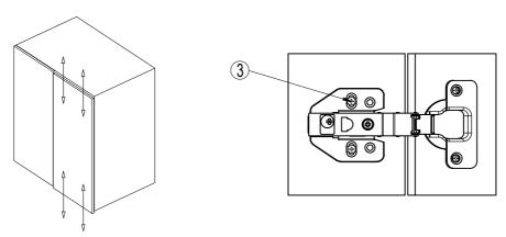
To adjust the height position of the door loosen the screws indicated on the side panel bracket, you will need to do this on all the brackets, adjust the door position and retighten the screws to secure the door.
