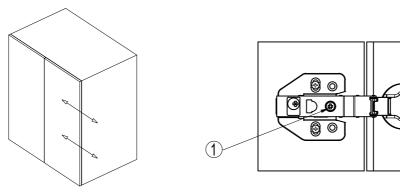
To move the door towards or away from the centre of the unit, loosen the screw shown. Adjust the position of the door then retighten the screw
