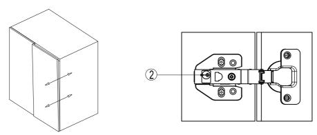
To move the door towards or away from the unit, adjust the screw indicated clockwise or anti clockwise to get the position required
